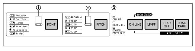
(1) FONT indicators: Press FONT. ② PITCH indicators: Press PITCH. ③ ON LINE indicator: Press ON LINE.
