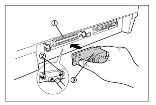
When connecting with a serial interface cable: Attach the serial interface cable (2) from your computer to the serial interface connector (1) and turn the screw clockwise to tighten.
