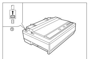
**3.** Raise the top cover (①). This is done by inserting the side pins of the top cover into the slots in the upper cabinet.
