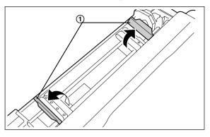
Place the paper with the printed side face down and align the paper sprocket holes (2) with the tractor pins (3), then close the tractor cover (1).
