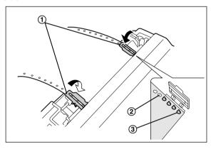
7. **1** Adjust the tractors (**1**) to remove any slack.
