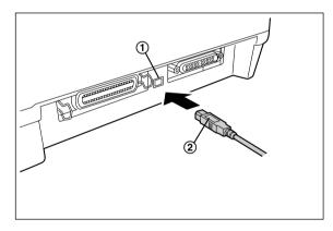
When connecting with a parallel interface cable: Attach the parallel interface cable (③) from your computer to the parallel interface connector (①) and secure the printer clips (②).
